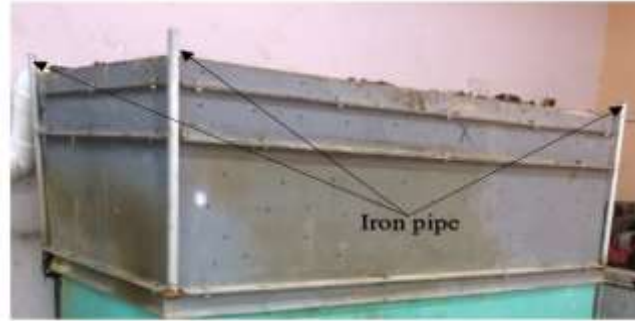
Figure 3: Iron Pipe Used to Install the Distribution Water Pipe.
